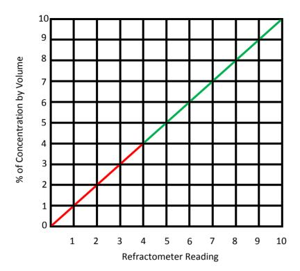
Dilution is too weak. Add 1 part concentrate with 10 parts water to increase concentration. Dilution is in correct range.
